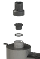
Pressure Test Cap Installation
